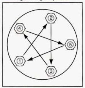
Tighten the wheel nuts firmly in a criss-cross sequence as shown. Turn the ratchet clockwise with the UP marking facing you.
